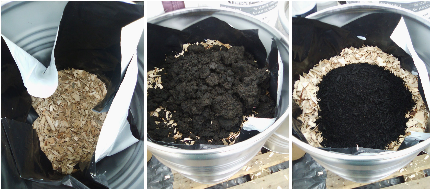
Mixing of 3 components: wood chips, sludge and biochar (from left to right)
