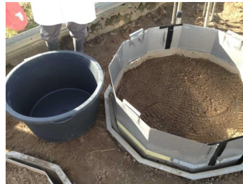
Application to outdoor soil lysimeter
